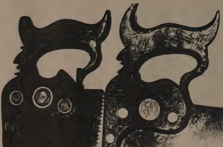
English saws. Left — Tillotson of Sheffield. Right — Ibbotson Peace & Co. Eagle Works. Most comfortable to hold.
